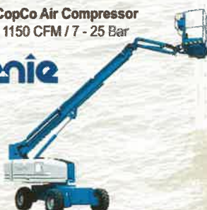
Boom Lift Working Height (6 - 41 Metres)
