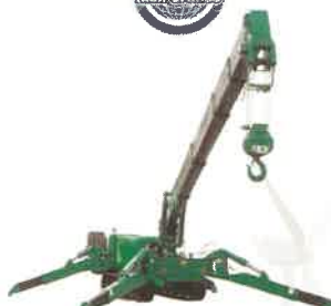
Mini Crawler Crane Lifting Capacity (1 - 6 Ton)
